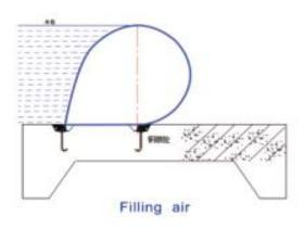
2) According to the slope, rubber dam is divided into pillow rubber dam and inclined rubber dam:
